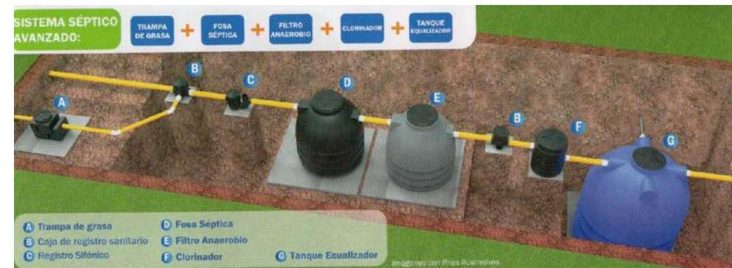
FIGURA 5.22. SISTEMA SÉPTICO AVANZADO.
