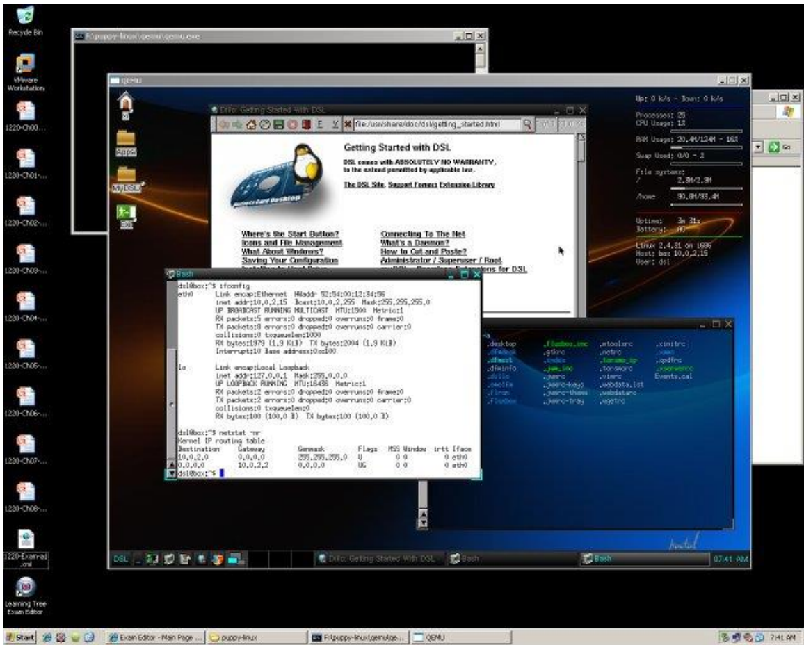
Figure 2. 14 Linux is running on top of QEMU on a Windows host.
