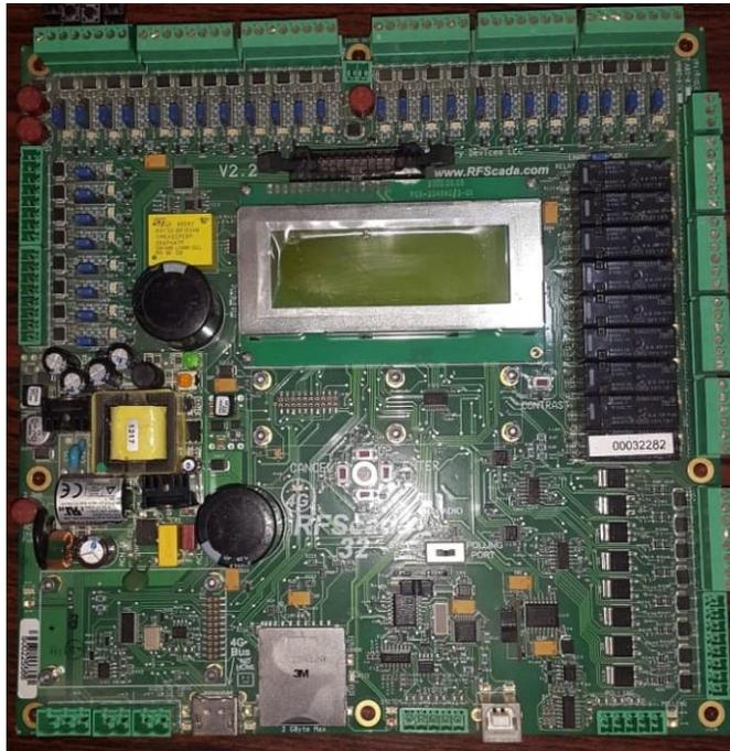
Figura A2.3: PLC RFScada 32
