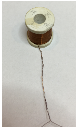
Figure 3.29: Constructed coil with twisted end.
