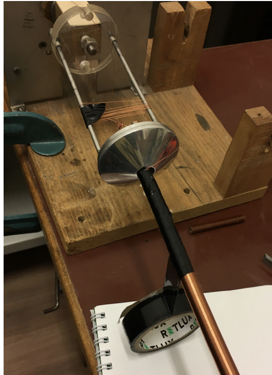
Figure 3.37: Rogowski coil with electric tape wrapping.
