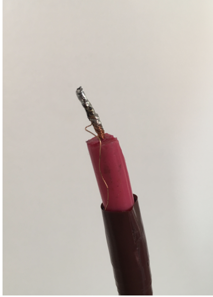
Figure 3.38: Welded ends of the Rogowski coil.
