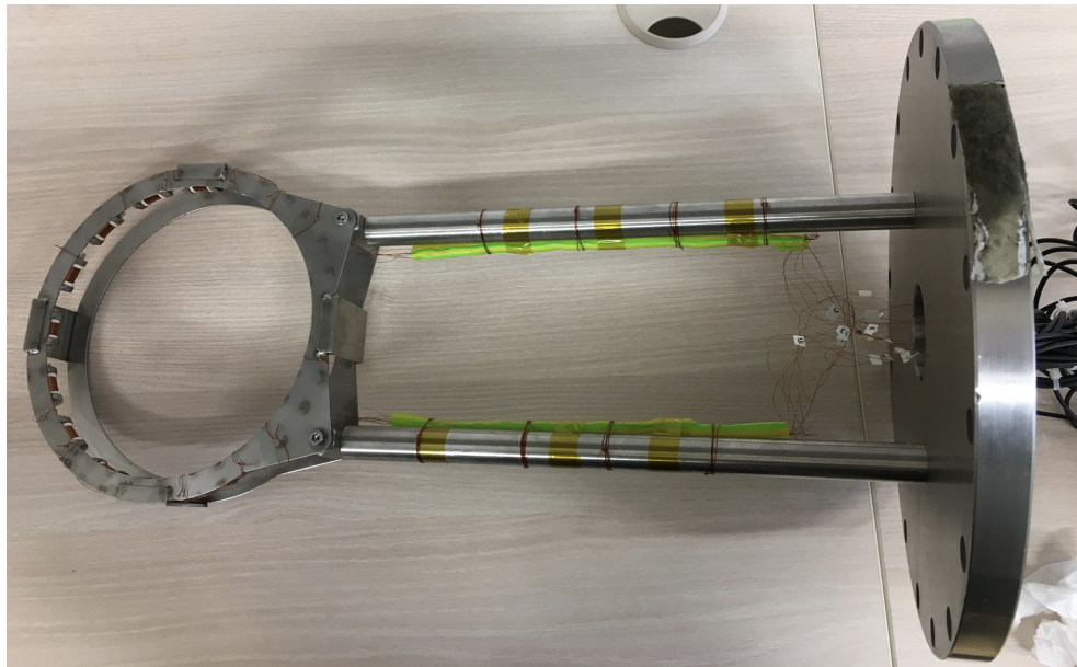
Figure 3.33: Complete assembly with 16 Mirnov coils installed.
