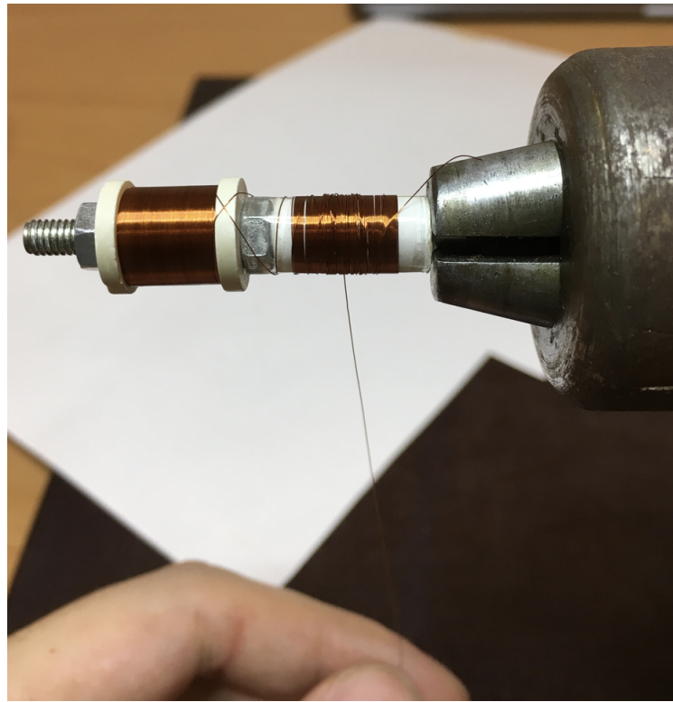
Figure 3.28: Coil and drill system for winding process.
