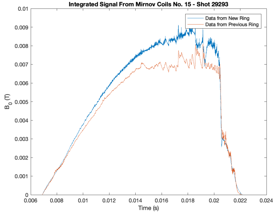
Figure 4.9: Signal integration comparison for coil 15 during shot No. 29293.
