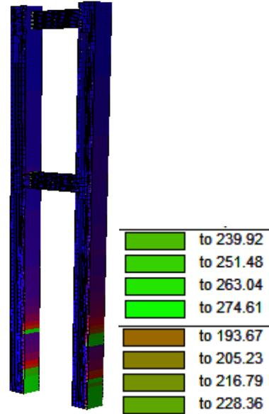
Figure 186. Stress in the reinforcement bars of the pushover, units in MPa. Software used: Augustus.
