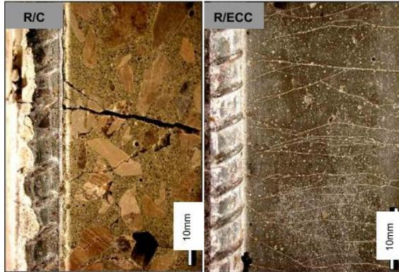
Figure 62. Compatible deformation between ECC and steel reinforcement (right) showing microcracking in ECC with load transmitted via bridging fibers. In contrast, the brittle fracture of concrete in normal R/C (left) causes unloading of concrete, resulting in high interfacial shear and bond breakage. Source: (V. C. Li, 2003)
