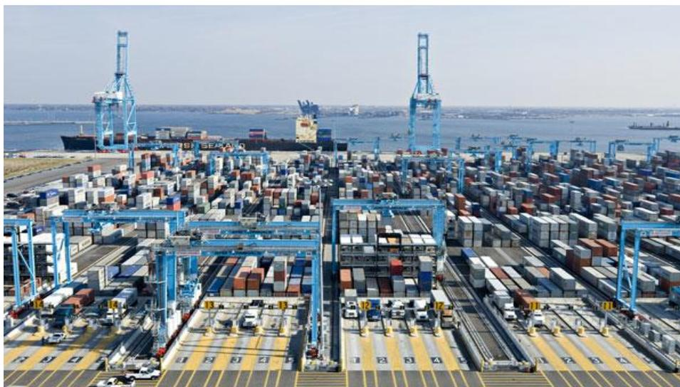
Figura 3.11 RTGs APM Terminals Virginia USA Fuente: APM Terminals [10]
