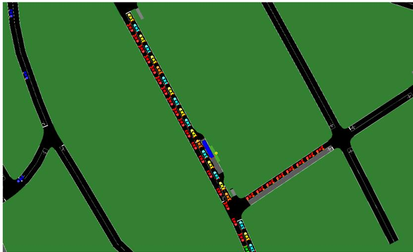
FIGURE 4.6: SUMO simulation view: bus stopping at bus-bay creating continuous flow of cars in the main road
