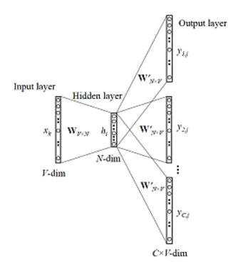
Figure 2. The skip-gram architecture. Obtained from [14]
