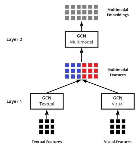
Figure 14. Proposed model for learning semantic representations with the help of Graph Convolutional Networks
