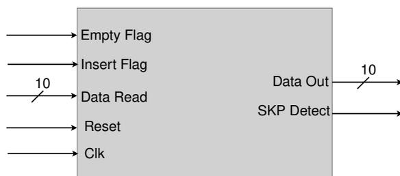
Figure 4.8: Block diagram of the Output Detect Unit of the Elastic Buffer for USB 3.0
