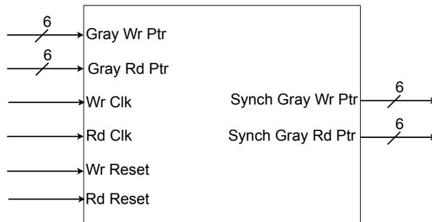
Figure 4.12: Simplified block diagram of Synchronizers for USB 2.0
