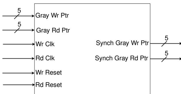
(a) Simplified block diagram of Synchronizers
