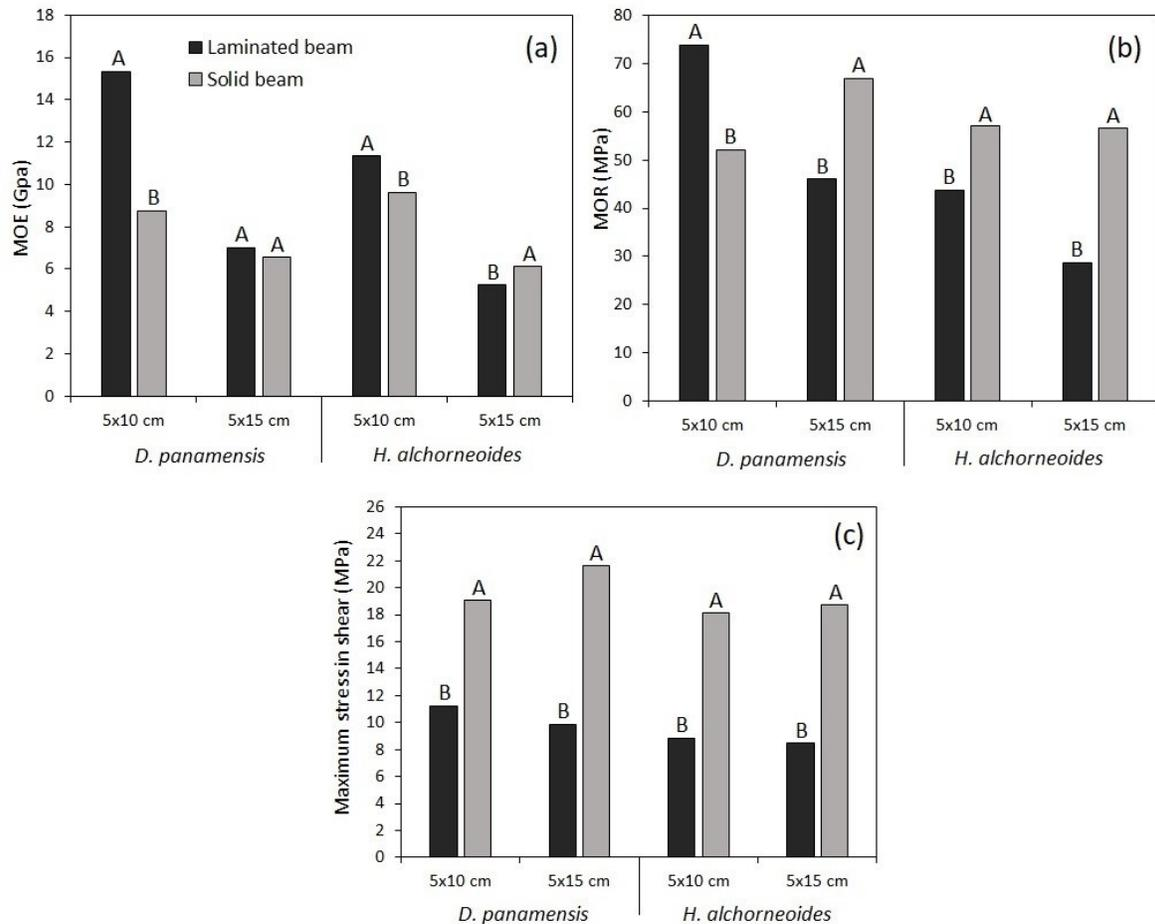
Figure 4. MOE (a) and MOR (b) obtained in the bending test and maximum stress in shear parallel to the grain (c) for glued laminated timber and solid timber beams built with *D. panamensis* and *H. alchorneoides* timber.
