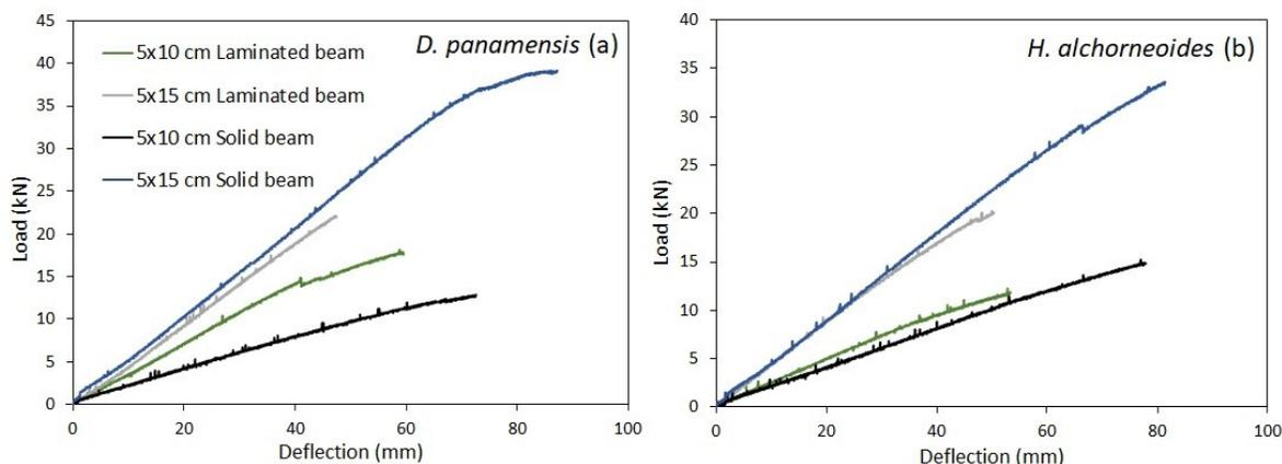
Figure 5. Average load versus deflection plots obtained in the bending test for glued laminated timber and solid timber beams built with *D. panamensis* and *H. alchorneoides* wood.
