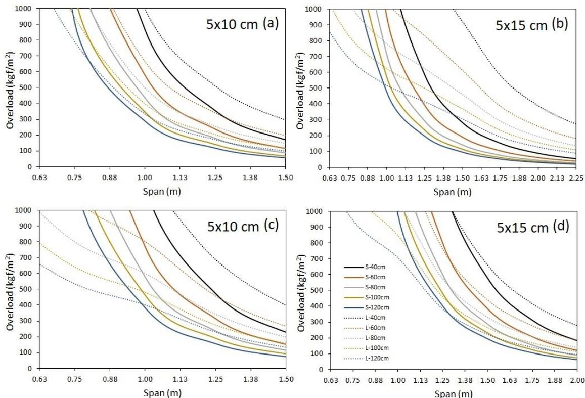
Figure 6. Overload vrs span for glued laminated timber and solid timber beams fabricated with *D. panamensis* (a and b) and *H. alchorneoides* (c and d) wood.
