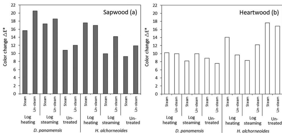
**Figure 3.** Color change in *D. panamensis* and *H. alchorneoides* lumber from different log treatments with and without steam application during drying.
