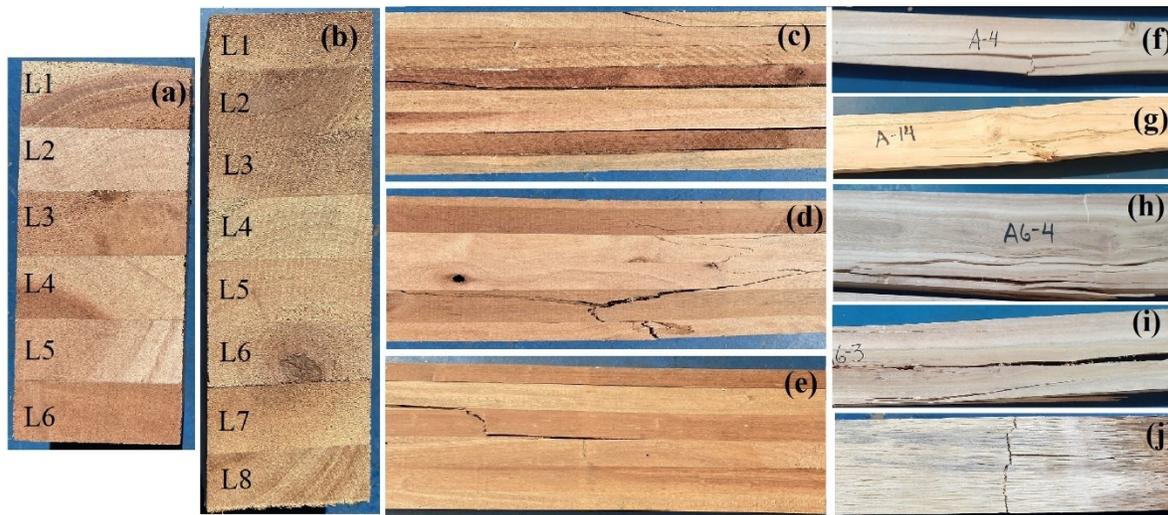
Figure 2. Number of laminates in glued laminated timber beams of 5 cm x 10 cm (a) and 5 cm x 15 cm (b), types of failures in glued laminated timber beams: delamination of glued line (c) and failure in lamina by tension (d) or shear (e), and failure in solid timber beams: simple tension (f), cross-grain tension (g), splintering tension (h), brash tension (i), and horizontal shear (j) in static bending.
