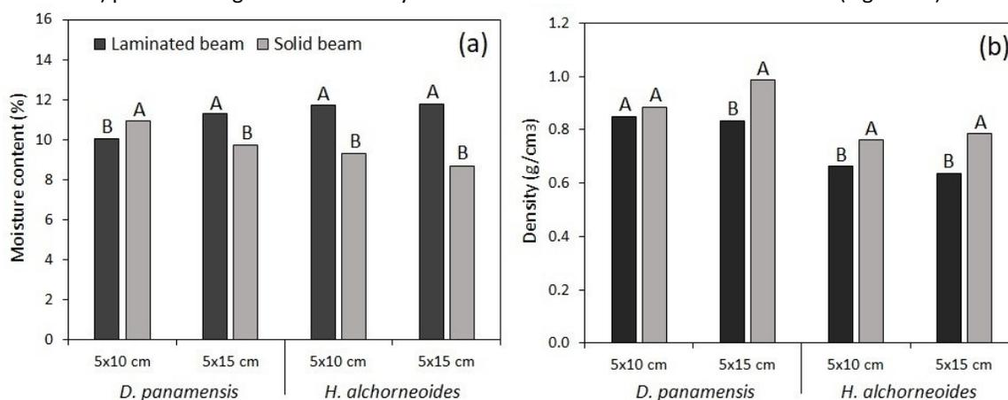
Figure 3. Moisture content (a) and density (b) for laminated and solid beams built with *D. panamensis* and *H. alchorneoides* timber.
