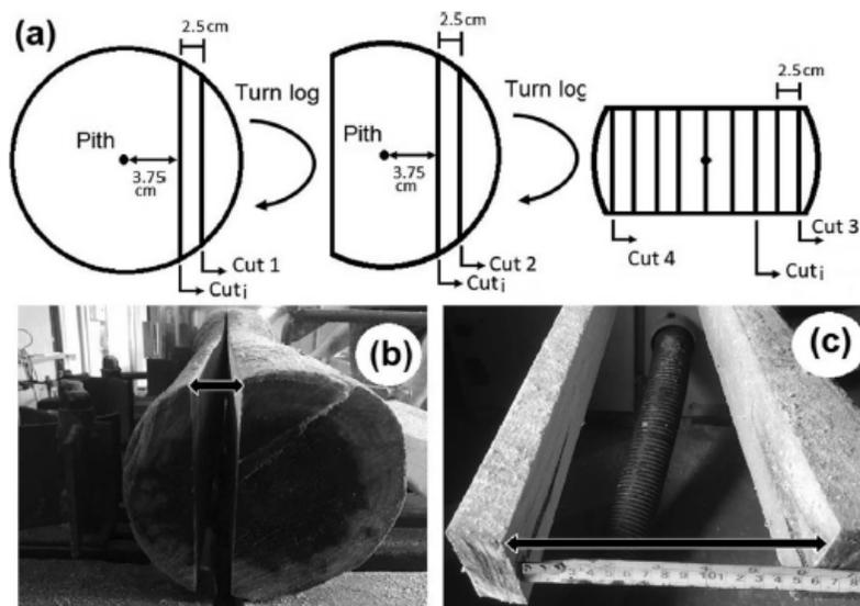
Figure 2.—Sawing pattern utilized in un-treated and heating and steaming for *Dipteryx panamensis* logs from a fast-growth plantation (a); crook due to sawing in sawlogs, (b) and crook due to sawing in semi-logs (c).
