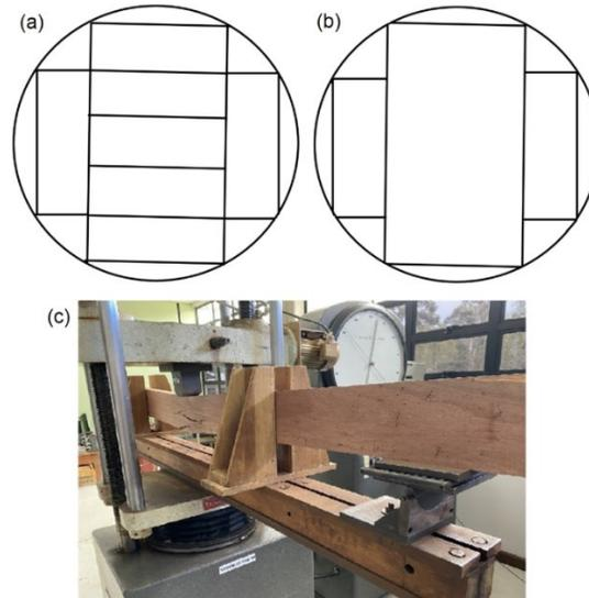
Figure 1. Sawing pattern utilized for obtaining 2.5 cm in thickness for fabricated glued laminated timber beams (a), sawing patten utilized for obtaining 6.2 cm thickness in solid timber beams (b) and bending test in three-point (c).
