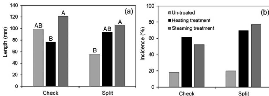
Figure 5.—Length (a) and incidence (b) of check and split defects in *Dipteryx panamensis* wood from a fast-growth plantation. Note: Different letters between treatments mean that there are statistical differences ( $P < 0.05$ ) between log treatments.
