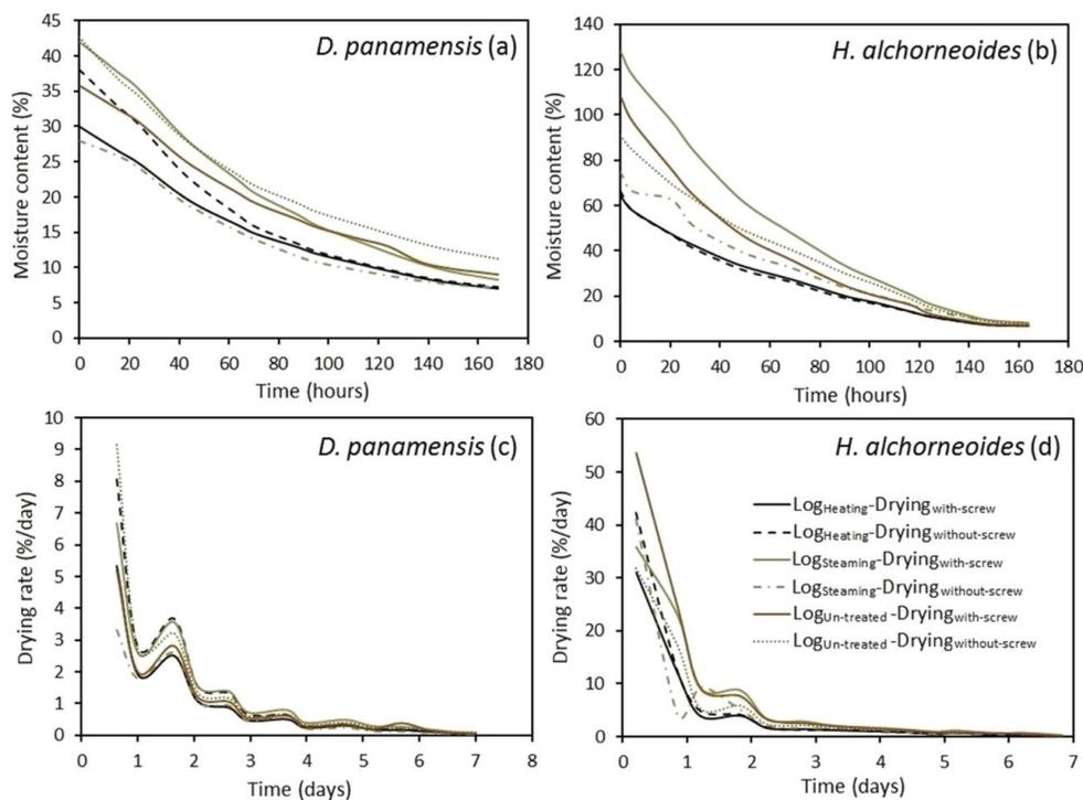
**Figure 2.** Variation of the moisture content and the drying rate in relation to time for *D. panamensis* (a and c) and *H. alchorneoides* (b and d) lumber with treatment.
