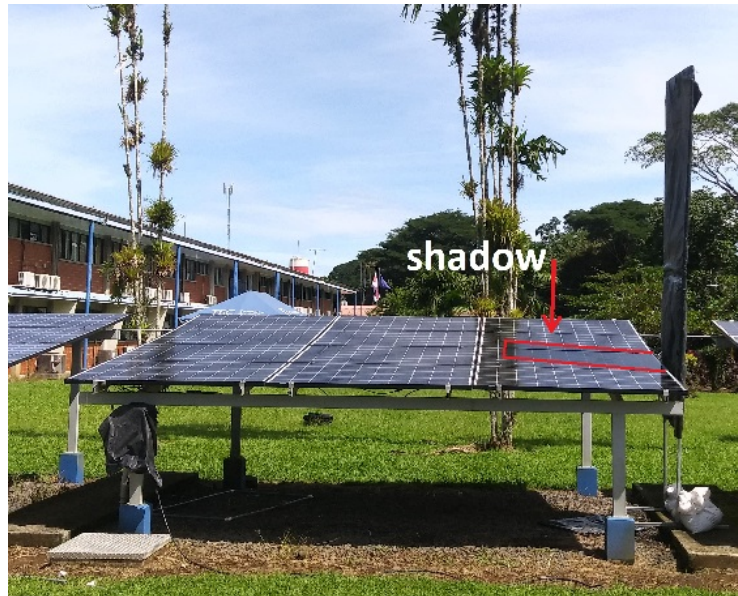
Fig. 9. Object used to generate the treatments of partial shade failures. The shadow generated corresponds to the PS1 treatment.
