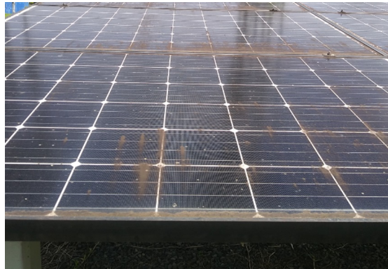
Fig. 2. Monocrystalline PV module analyzed with the presence of natural non-uniform dirt.
