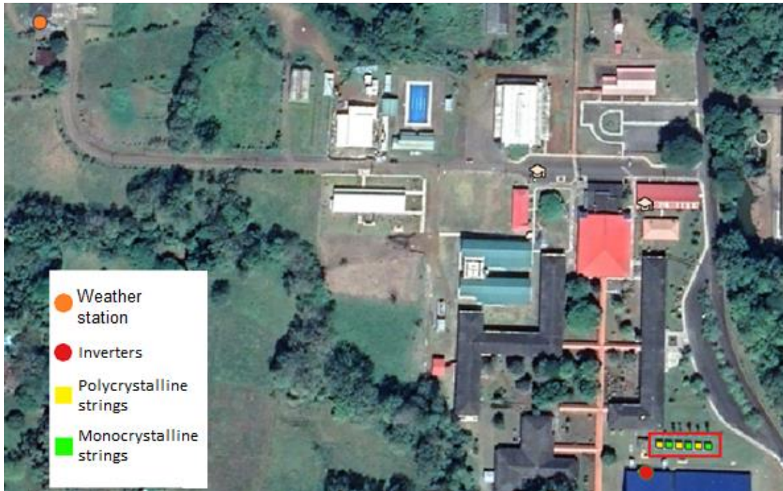
Fig 10. Aerial photograph with the location of the parts of the PV installation in San Carlos. The PV strings are enclosed in a red box. Image taken and adapted from Google Earth.
