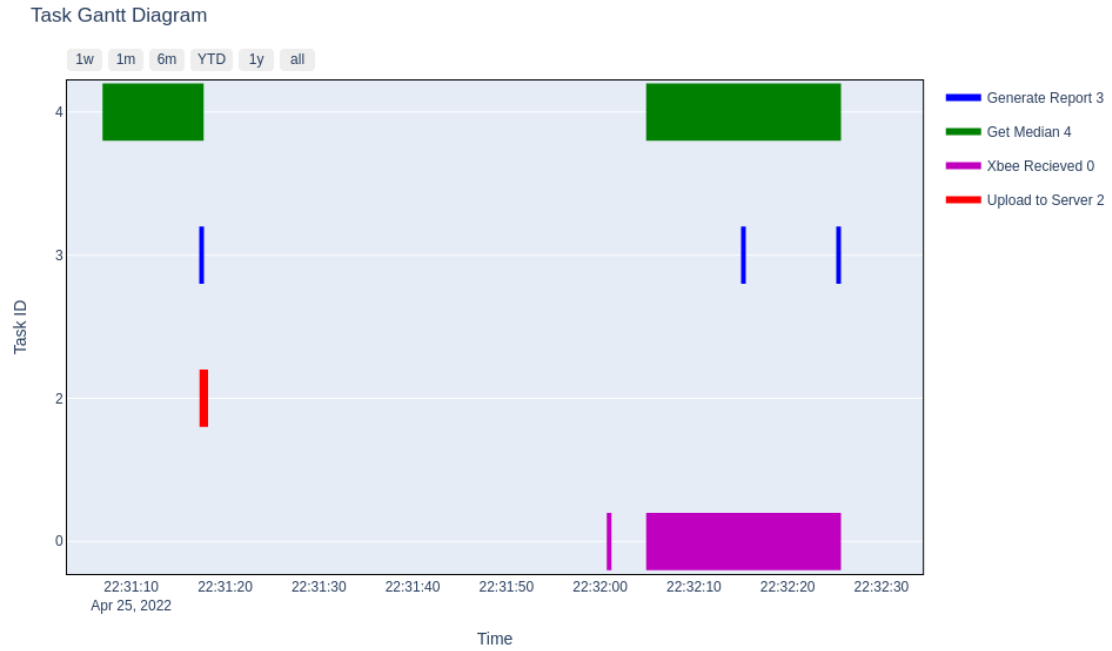
Figure 4.2: Tasks Gantt plot eBridge 2019 code running as master/primary sensor node running in eBridge 2021 HW with RPI3 B+ with f = 1.4 GHz. Details of the test in table 4.1
