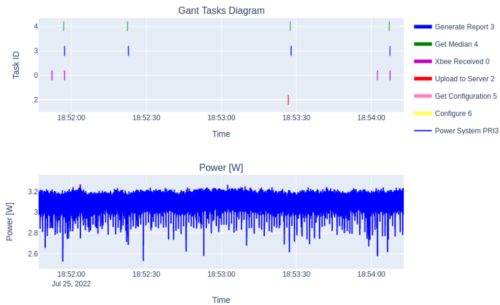
Figure 6.5: Tasks Gantt Plot vs Power (W) of eBridge 2021 code running as master/primary sensor node running in eBridge 2021 HW with RPI3 B+ with f = 1.4 GHz. Details of the test in table 6.1
