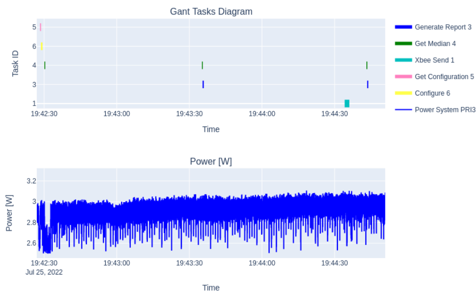
Figure 6.11: Tasks Gantt Plot vs Power (W) of eBridge 2021 code running as a slave/secondary sensor node running in eBridge 2021 HW with RPI3 B+ with f = 1.4 GHz. Details of the test in table 6.7
