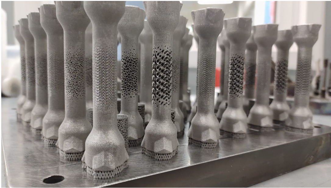
Figure 3.5.: DLMS fabricated compression and fatigue test specimens [2]
