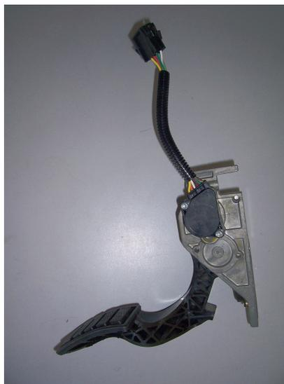
EDC accelerator pedal assembly ©Panoha, CC BY-SA 3.0
