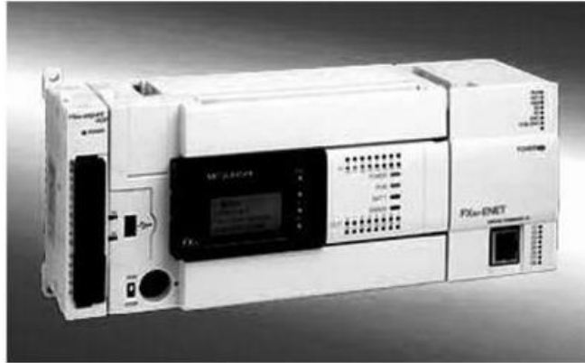
Figura 3.9. PLC Compact Mitsubishi: MELSEC FX3U (Bolton, W. 2009)
