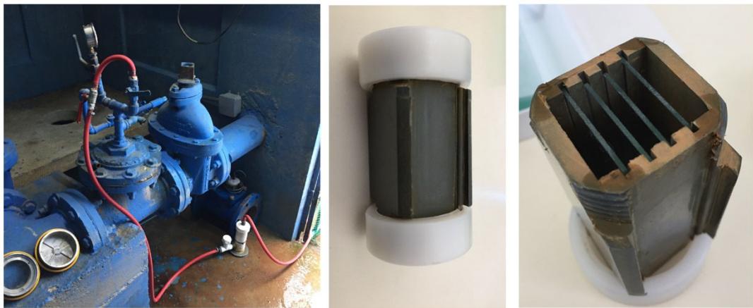
Figure 3-2. Flow cell device to collect bacteria from groundwater systems for microscopic examination.
