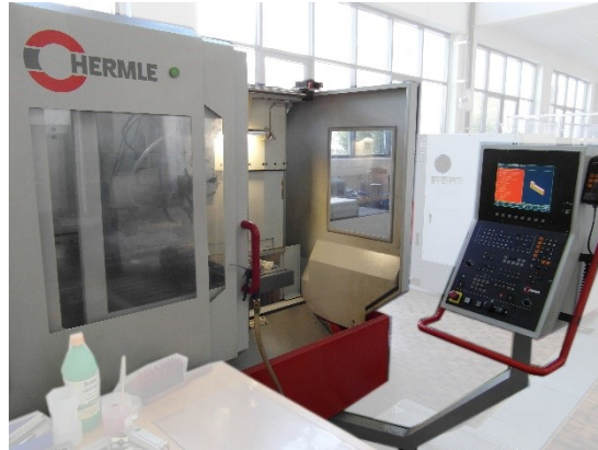
Figure 1.1: CNC milling machine Hermle UWF900E. Source: [4]
