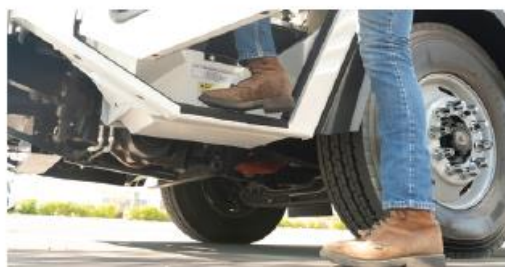
True low entry 18" step-in height on both sides
