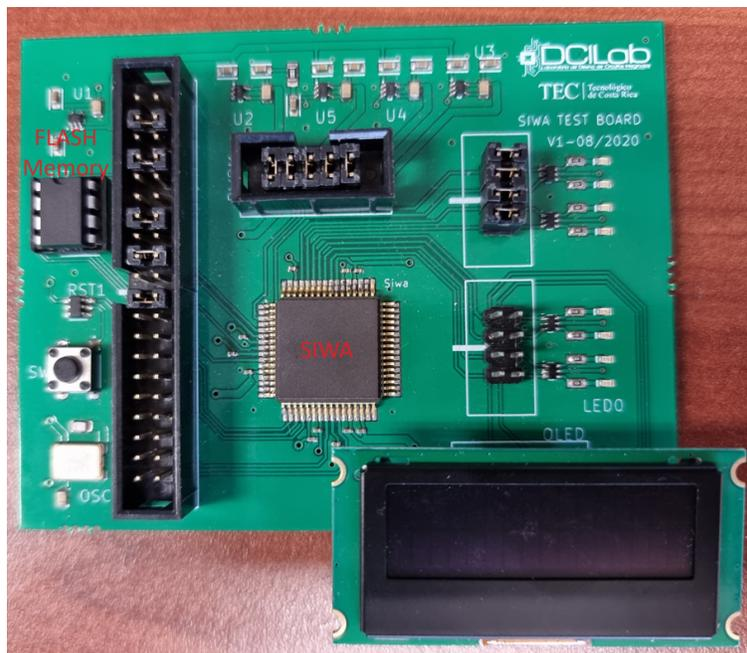
**Figure 4.12.** SIWA on PCB with other discrete components.
