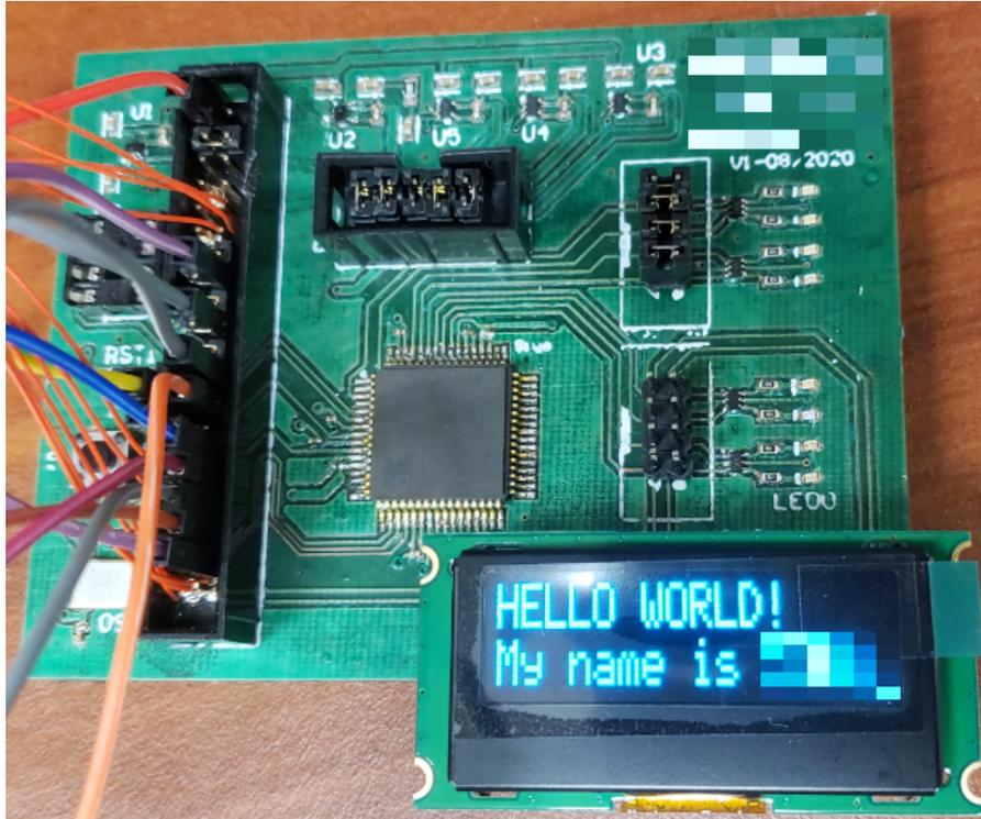
**Figure 4.9.** "Hello World" program on a OLED display, emulating the required I<sup>2</sup>C protocol via software routines and the GPIO ports.
