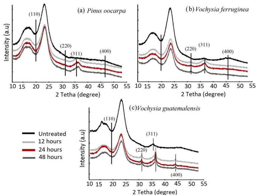
**Figure 3.** X-ray diffraction (XRD) in untreated wood and magnetic wood of three tropical wood species from fast-growth plantations in Costa Rica: (a) *Pinus oocarpa*, (b) *Vochysia ferruginea* and (c) *Vochysia guatemalensis*.
