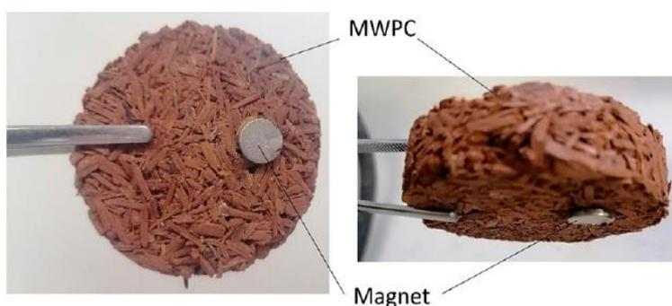
Figure 6. A magnetized sample of magnetic wood particleboards composite (MWPC) for *Pinus oocarpa*, attracted by a magnet.
