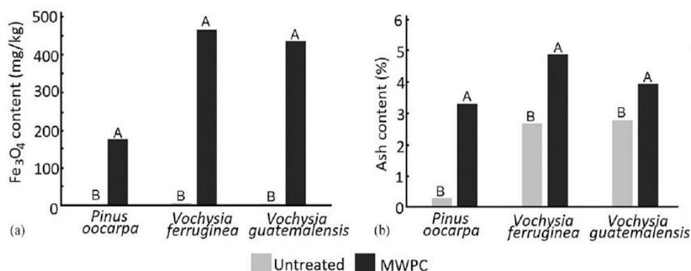
Figure 2. Fe<sub>3</sub>O<sub>4</sub> (a) and Ash (b) content of magnetic wood particleboards composite (MWPC) of three tropical species from fast-growth plantations in Costa Rica. Note: Uppercase letters mean statistical differences between treatments at 95% significance.
