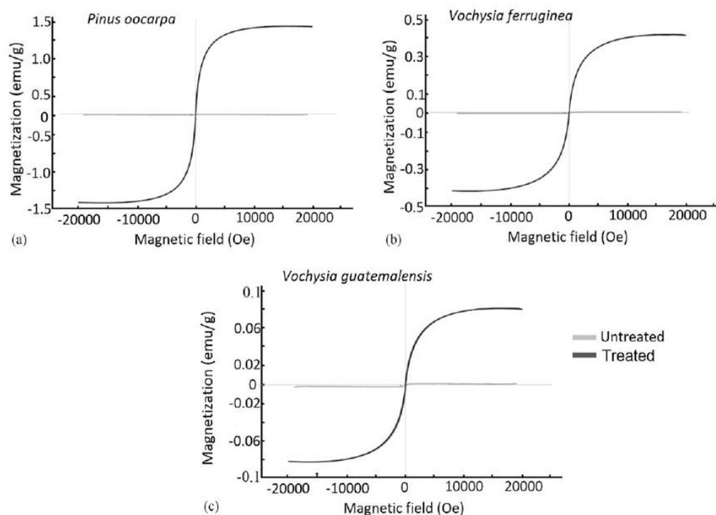
Figure 5. Magnetic hysteresis curves of three magnetic wood particleboards composite of tropical species (a-c) from fast growth plantations in Costa Rica.
