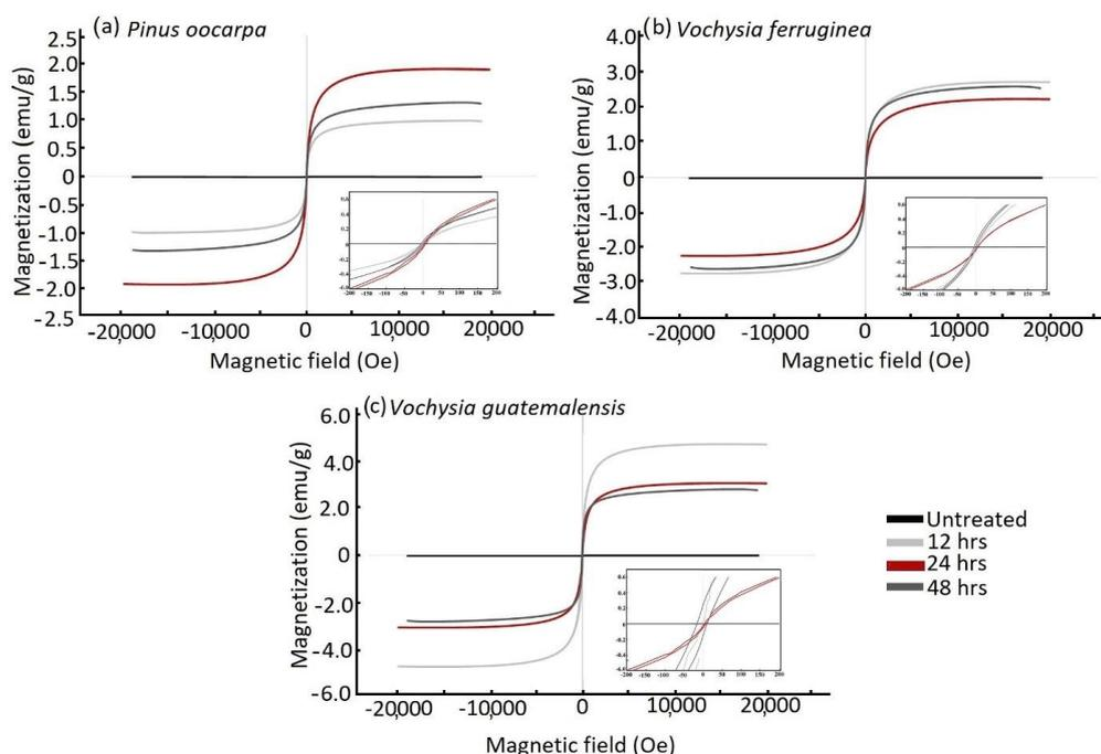
**Figure 5.** Magnetic hysteresis curves of untreated wood and magnetic wood with three different immersion times in ammonia in three tropical wood species from fast-growth plantations in Costa Rica: (a) *Pinus oocarpa*, (b) *Vochysia ferruginea* and (c) *Vochysia guatemalensis*.
