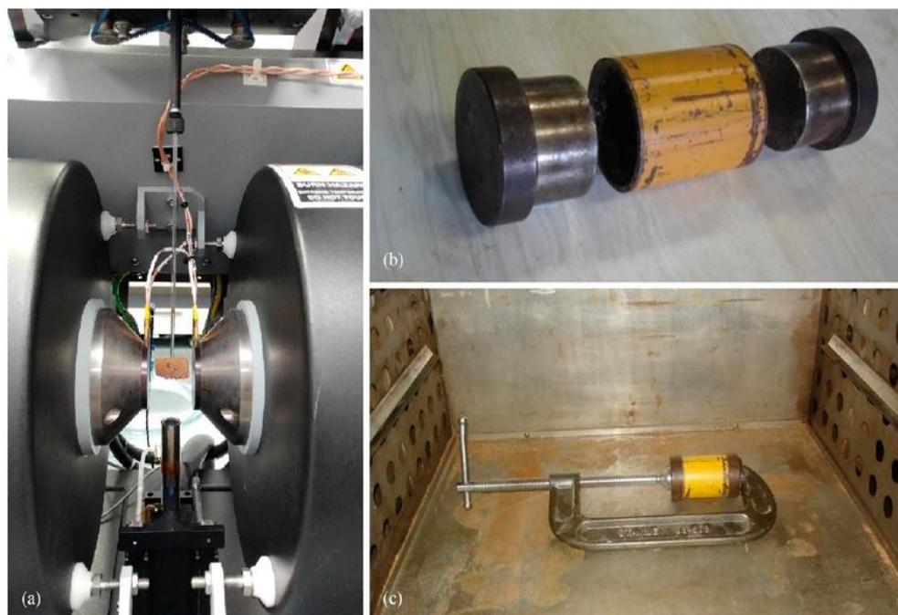
Figure 1. Vibrating sample magnetometer and location of composite sample (a), metal rack utilized (b), and press application during heating in the particleboards fabrication (c).
