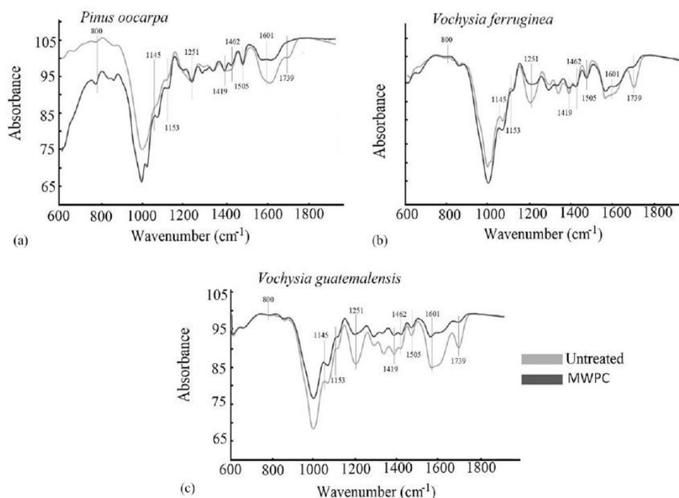
Figure 3. Fourier transform IR spectrum of magnetic wood particleboards composite (MWPC) of three tropical species (a-c) from fast-growth plantations in Costa Rica. a) *Pinus oocarpa* b) *Vochysia ferruginea* c) *Vochysia guatemalensis*. Note: Super-script letters mean statistical differences between treatments at 95% significance.
