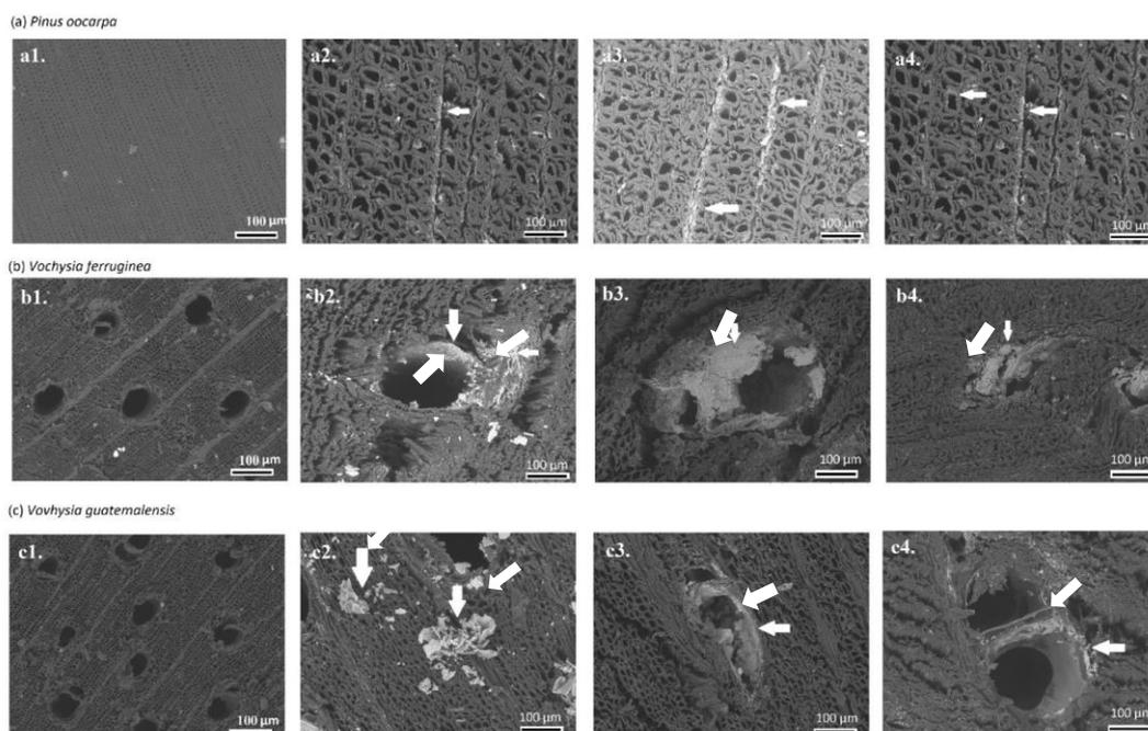
**Figure 2.** Scanning electron microscope (SEM) images showing  $\text{Fe}_3\text{O}_4$  NPs formation of magnetic wood with three different immersion times in ammonium (1: untreated, 2: 12 h, 3: 24 h; 4: 48 h) in three tropical wood species (a–c) from fast-growth plantations in Costa Rica. Note: The white arrow indicates the formation of  $\text{Fe}_3\text{O}_4$  NPs in the rays, fibers or vessels.
