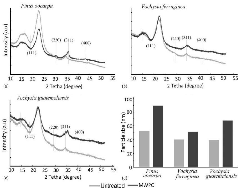
Figure 4. X-ray diffraction of magnetic wood particleboards composite (MWPC) (a-c) and particle size of  $\text{Fe}_3\text{O}_4$  of three tropical species (d) from fast-growth plantations in Costa Rica.
