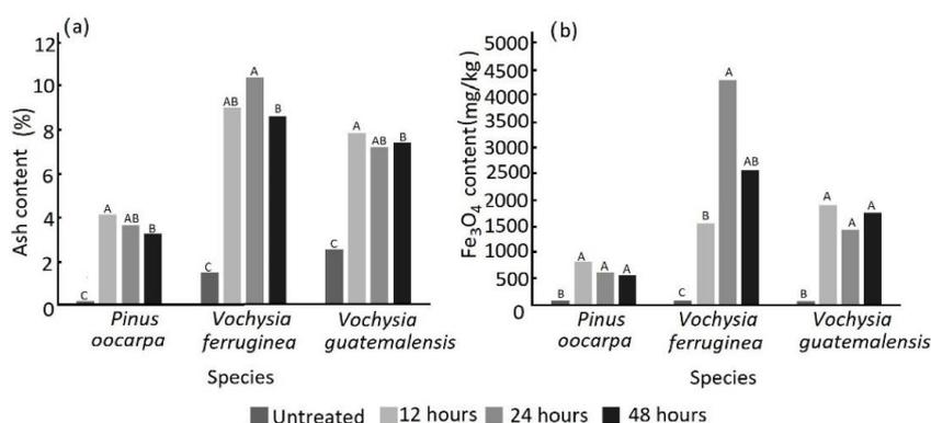
**Figure 1.** Ash (a) and Fe<sub>3</sub>O<sub>4</sub> NPs (nanoparticles) (b) content of untreated wood and magnetic wood with three different immersion times in ammonia in three tropical wood species from fast-growth plantations in Costa Rica. Note: Letters mean significant differences between treatment at 95% in each species.
