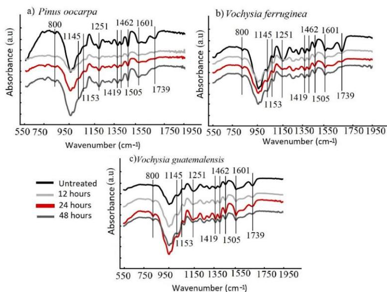
**Figure 4.** Fourier transform infrared spectroscopy (FTIR) spectrum of untreated and magnetized wood with three times of three tropical wood species (a–c) from fast-growth plantations in Costa Rica: (a) *Pinus oocarpa*, (b) *Vochysia ferruginea* and (c) *Vochysia guatemalensis*.
