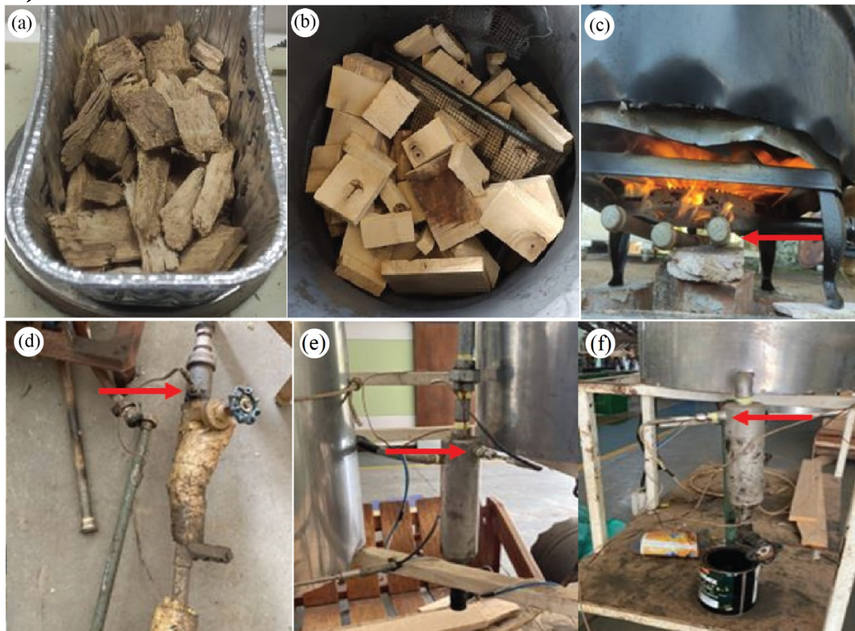
Figure 1. Wood residues of G. arborea used in the pyrolysis process: (a) chip parentwood and (b) board-ends solid parentwood. Different parts in the reactor: Non-condensable gases outlet (c) and temperature meter probes at three stages of the wood residues pyrolysis process: pyrolizer gas outlet (d), after the first cooler (e) and after the second cooler (f).
