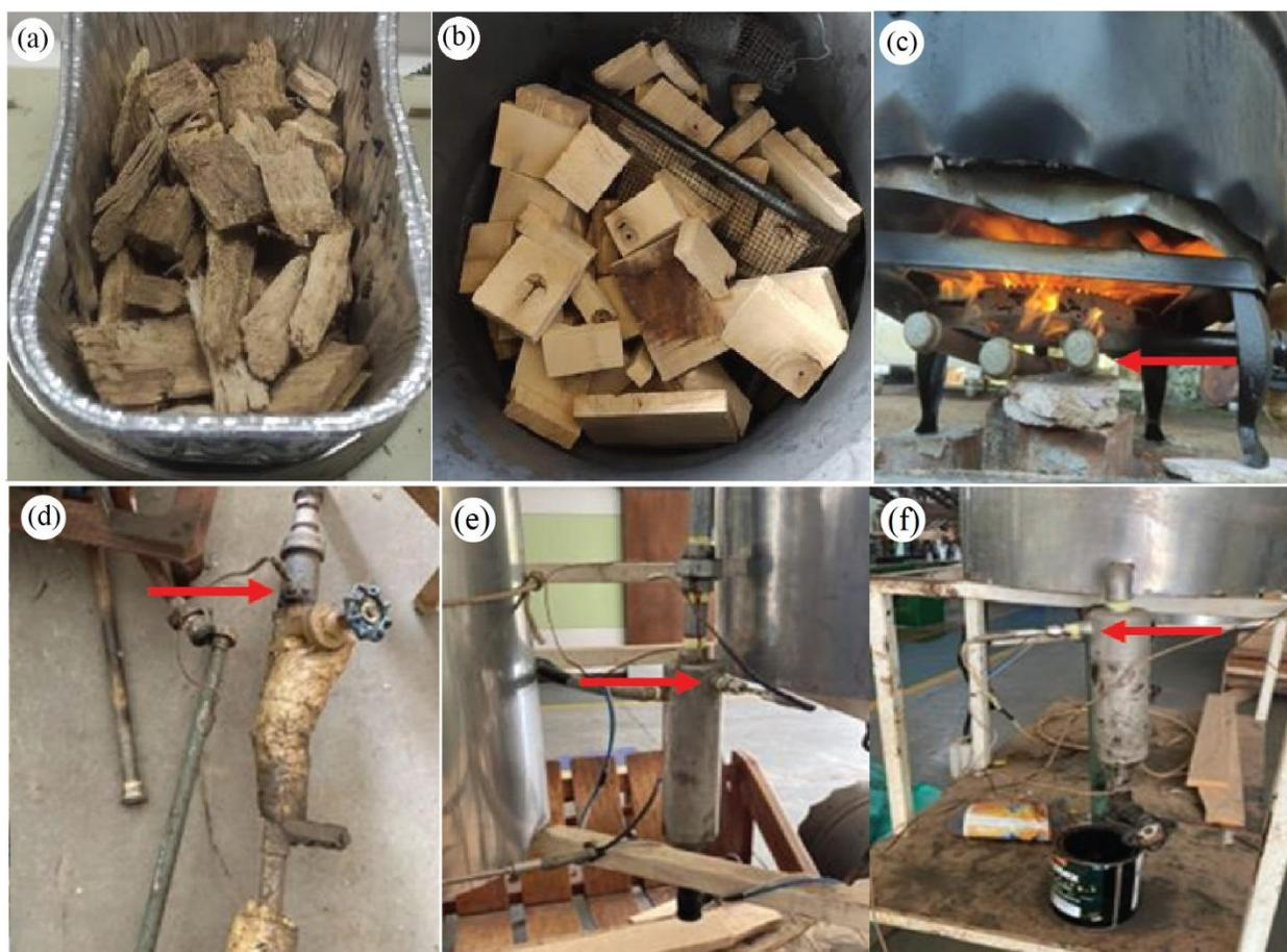
**Figure 1.** Wood residues of *G. arborea* used in the pyrolysis process: chip parentwood (a) and board-ends solid parentwood (b). Different parts in the reactor: Non-condensable gases outlet (c) and temperature meter probes at three stages of the wood residues pyrolysis process: pyrolyzer gas outlet (d), after the first cooler (e) and after the second cooler (f).
