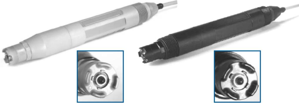
Hach Digital pH/ORP sensors are available in convertible (PEEK® or Ryton®), insertion, and sanitary body styles. Three electrodes are used in these sensors to increase measurement accuracy and eliminate sensor ground loops.
