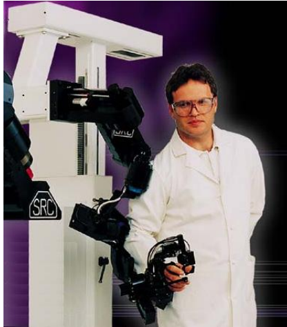
Figura 3.13 Exoesqueleto fijo (Dextrous Hand Master Exoskeleton). [11]
