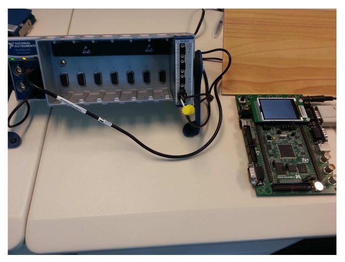
Figure E.1: Connection scheme of the hardware for the current acquisition.
