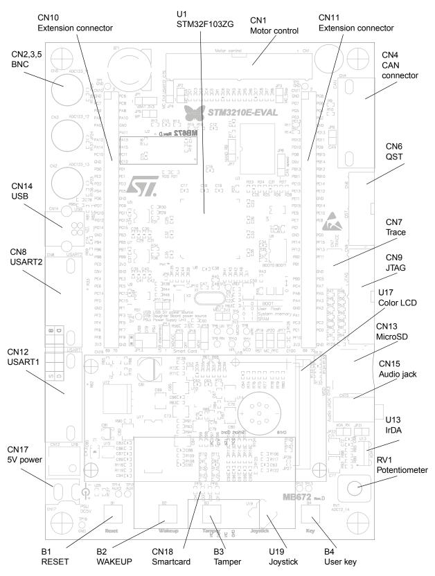
Figure 1.2: STM3210e-eval evaluation board layout.
