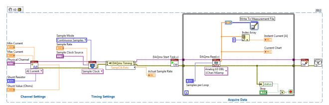
Figure D.1: LabVIEW block diagram (source code).
