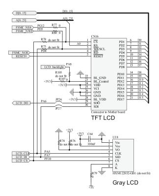
Figure 2.2: Schematic of the TFT LCD in the STM3210e-eval board [13].
