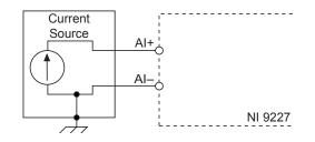
Figure 2.5: Connecting a Grounded Current Source to the NI 9227 [6]
