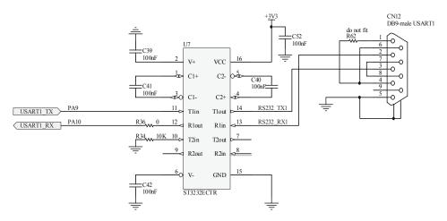
Figure 2.3: Schematic of the USART in the STM3210e-eval board [13].
