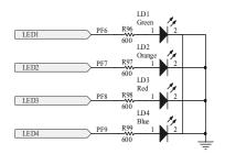
Figure 2.4: Schematic of the LED's in the STM3210e-eval board [13].
