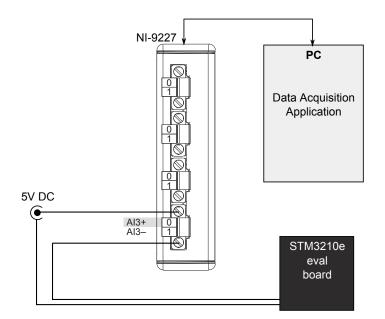
Figure 4.10: Schematic of the STM3210e-eval board and the acquisition system.
