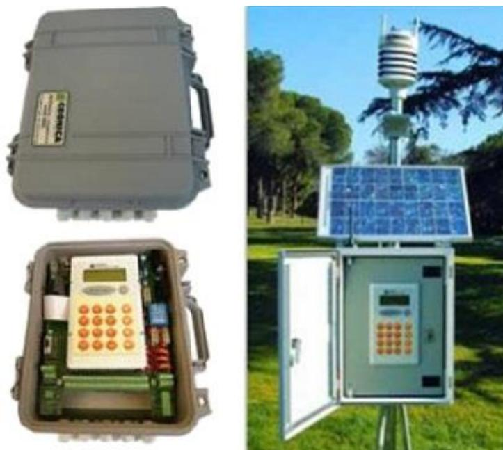
**Figura 4.4** Datalogger METEODATA-HYDRODATA-3000C de GEONICA.
