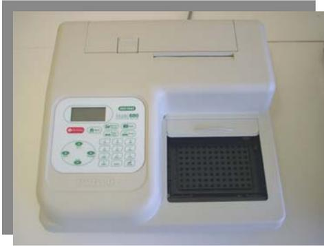
**Fig. 1.** Microplate Reader
