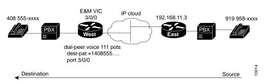
Figure 20 Linking PBXs over the IP Network (Local Dial Peers)
