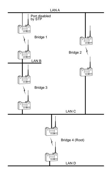
If there is heavy traffic between LAN A and LAN B, it would be more efficient to have Bridge 1 become the root with the port on Bridge 3 being disabled.
