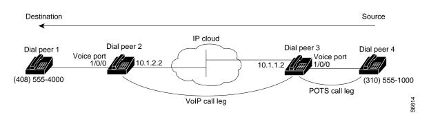
To complete the end-to-end call between dial peer 1 and dial peer 4 as illustrated in Figure 2-6, enter the following commands on router 10.1.1.2:
