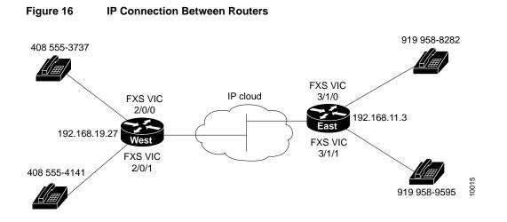
Look at the connection between the West router and the IP network. This connection does not include a voice port or an attached telephone—it leads from a WAN interface to a remote destination somewhere on the IP network. IP routers know how to locate IP addresses on the network, but they do not know how to locate telephone numbers. To route an outgoing voice call over this connection, the West router has to associate a telephone number in the East office with the IP address of the East router.
