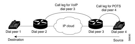
These 2 call legs are associated by the connection ID. The connection ID is global across the voice network, so that you can associate 2 call legs on one router with 2 call legs on another router, thereby providing an end-to-end view of a call.
