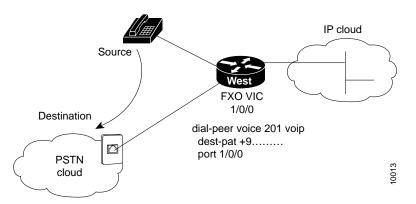
To create a local (POTS) dial peer for an FXS interface, as explained earlier, you enter the complete telephone number of the attached telephone as the destination pattern for incoming calls. When you create a local dial peer for an FXO interface, however, the destination pattern refers to outgoing calls, and you can include wild cards in it, because the PSTN performs the switching.
