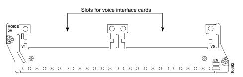
To install a voice network module, slide it into a slot in the router chassis (Figure 3). Use a number 1 Phillips or small flat-blade screwdriver to fasten the module's mounting screws.
