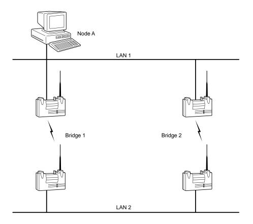
If Node A transmits a multicast packet, both Bridge 1 and Bridge 2 will try and forward the packet to LAN 2. Each bridge, on seeing the other's transmission on LAN 2, will forward the packet back to LAN 1. The cycle will continue and the packet will loop forever taking up all of the bandwidth of the bridges.
