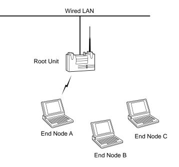
As another example, suppose you only wanted to block End Node C and did not care about any other nodes. In this case you would leave auto-association "On" and add a static entry for End Node C to block it.
