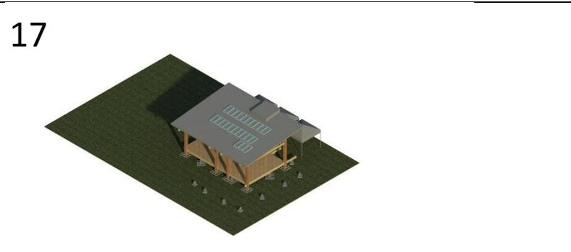
Placement of the roof components (Solar panels, water collectors and solar chimney)
