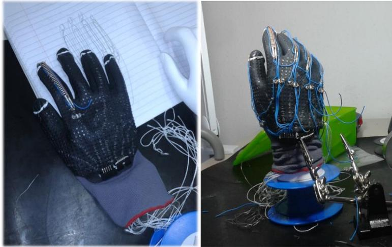
**Figure 6-3.** Assembly of the Electronic Layout of the Glove
