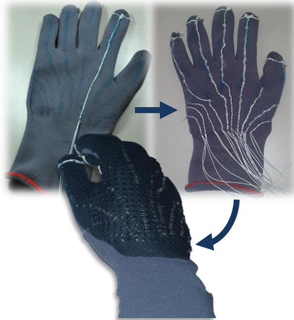
**Figure 6-2.** Assembly of the Tendon Layout of the Glove
