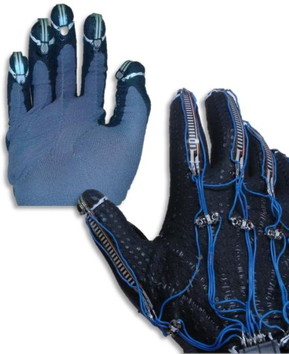
**Figure 6-4.** Electronic Layer of the Glove
