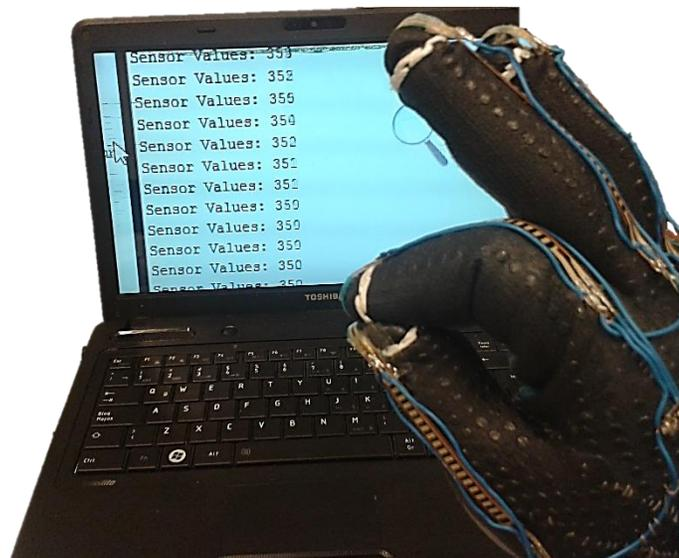
**Figure 6-12.** Characterization of the force sensor
