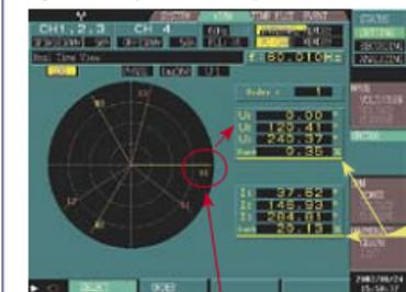
Display the fundamental voltage waveform for the 1st order (U1, U2, and U3) as a phase angle of 360° as a standard. Ideal for checking three-phase power lines.
