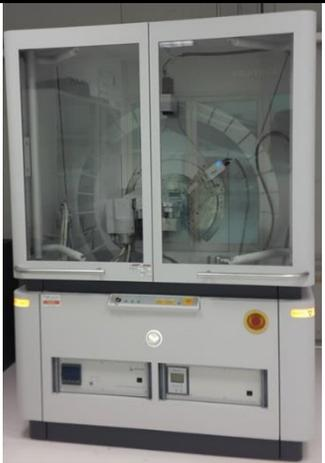
A photograph of an X-ray diffractometer. It is a large, white, industrial-looking machine with a glass-enclosed upper section containing the goniometer and a control panel with a screen and buttons on the lower section. | Difracción de rayos<br>X |
