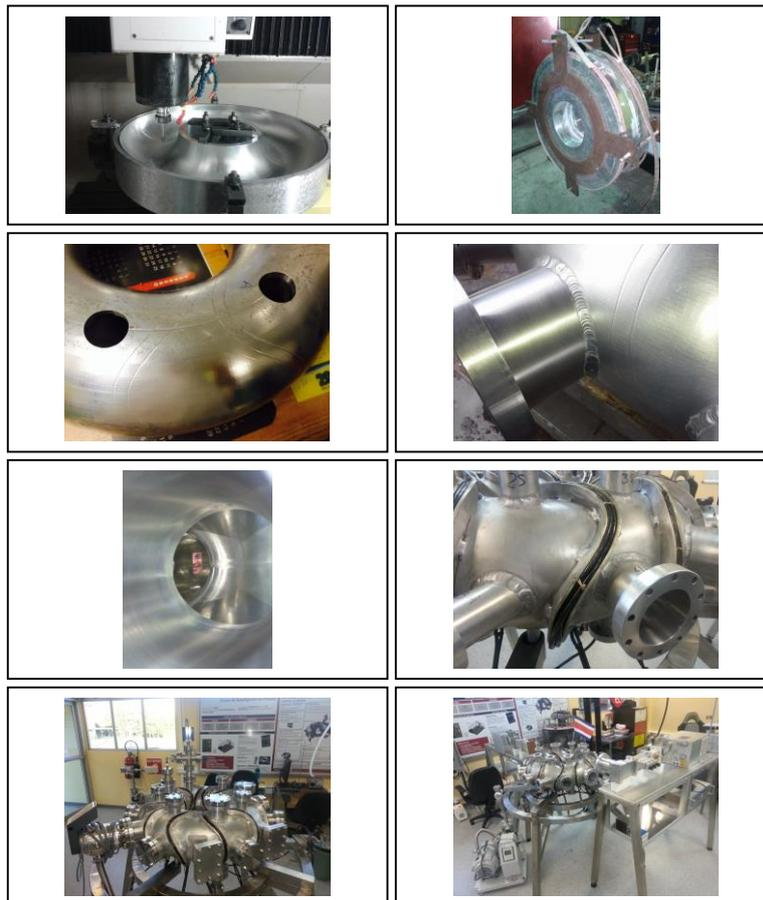
**Figure 2. Stages of the vacuum vessel construction.**
