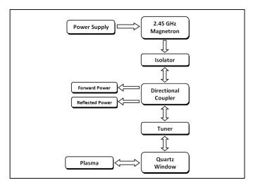
Figure 6. Simple block diagram of the Heating System of the SCR-1.
