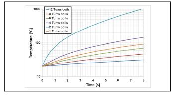
Figure 3. Temperature comparison between different coils configurations.
