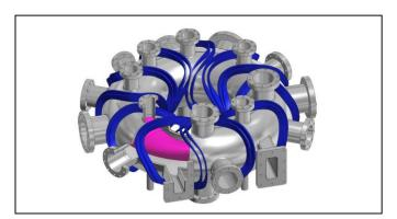
Figure 1. SCR-1 vacuum vessel drawing.
