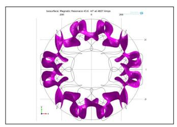
Figure 11. Resonant surface (2.45 GHz) for I=4607 A.
