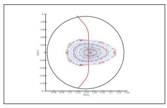
Figure 9. Magnetic surfaces at  $\Phi = 0^{\circ}$ .
