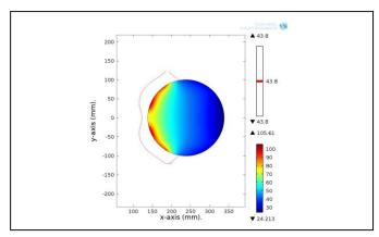
Figure 10. Contour map of magnetic field at  $\Phi$  =  $0^{\rm o}$  for I=4607 A.
