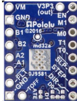
Figure 7.1: Driver for the stepper motors.
