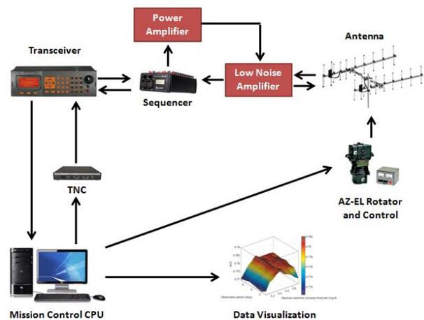
Fig. 8. Block diagram of Irazú ground segment.
