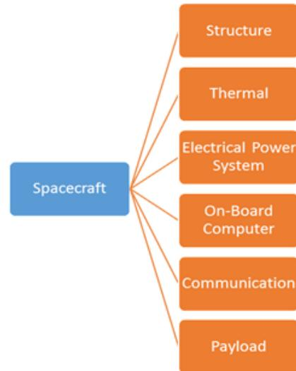
Fig. 5. Irazú CubeSat subsystems.
