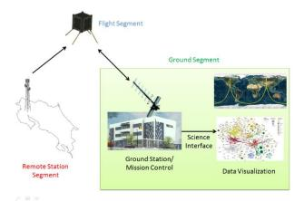
Fig. 4. Irazú project concept of operations.
