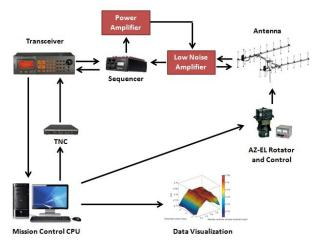
Fig. 8. Block diagram of Irazú ground segment.
