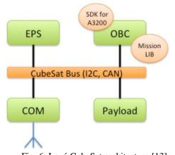
Fig. 6. Irazú CubeSat architecture [13].
