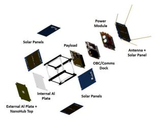
Fig. 7. Irazú CubeSat exploded view.
