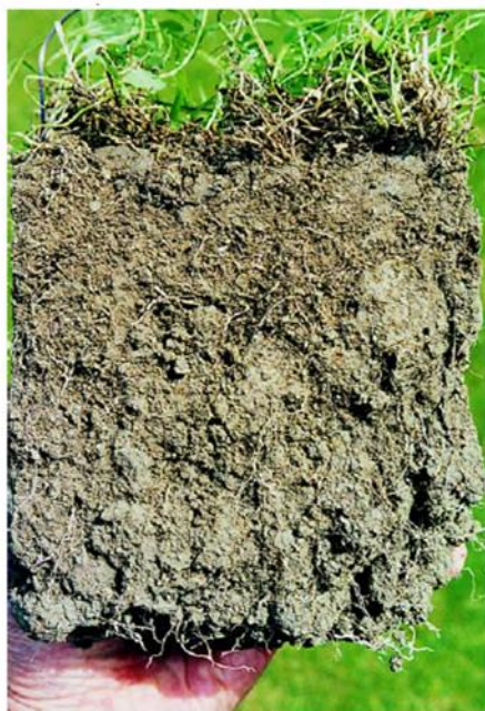
MODERATE CONDITION VS = 1 Soil macropores between and within aggregates have declined significantly but are present on close examination of clods showing a moderate amount of consolidation
