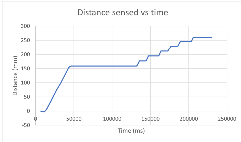
Figure 4.27: Distance output when in typical usage in position 2 stopping at positions 156 mm, 171 mm, 185 mm, 200 mm, 216 mm, 231 mm and 243 mm
