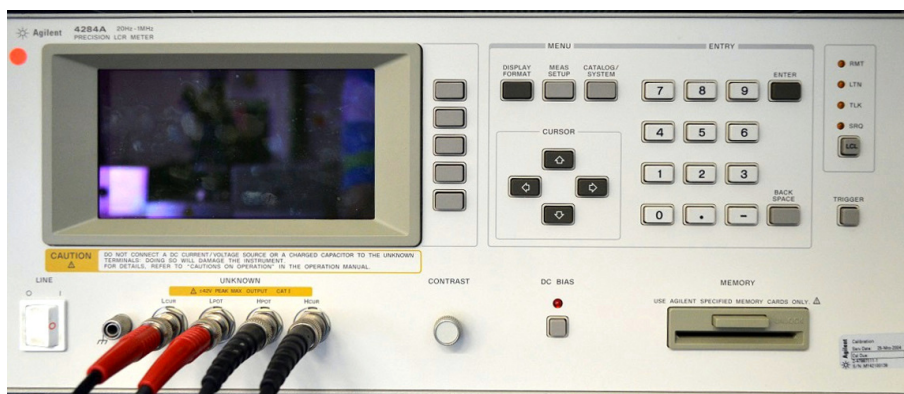
Figure 41: Agilent 4284A LCR meter for performing the EIS characterization.
