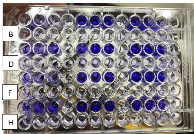
Figure 7. Top view of a 96-well microtiter plate filled with 200 µL of 96% ethanol. Rows B, D, F and H acted as controls, as did the wells in the middle of each triplicate sample.
