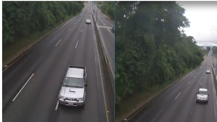
(b) Geometric variance - The car varies its shape when it gets closer to the camera
