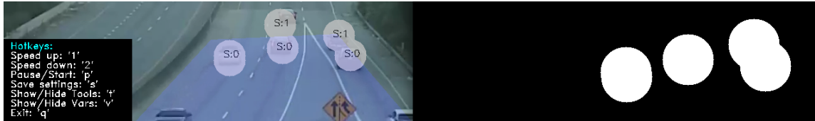
Figure 3.8: Black map (on the right) based on the frame (on the left) of a vehicle with two false-positives
