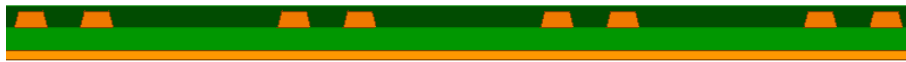
Figure 3.12: Section of the 2D MR model with a length in the outsider lines of 50 mil in each side
