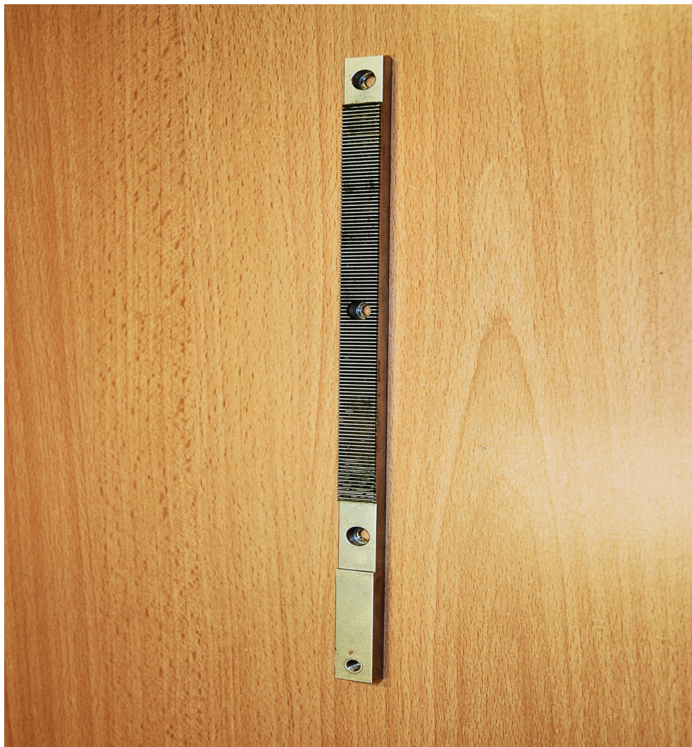
Figure B.1: Rack on the rail of GRACE system, with a different resolution than the lead screw, it was a cause of interference.
