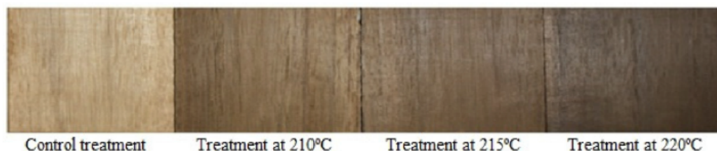
Figure 2. Color changes in the thermally-treated teak wood, at three different temperatures.
