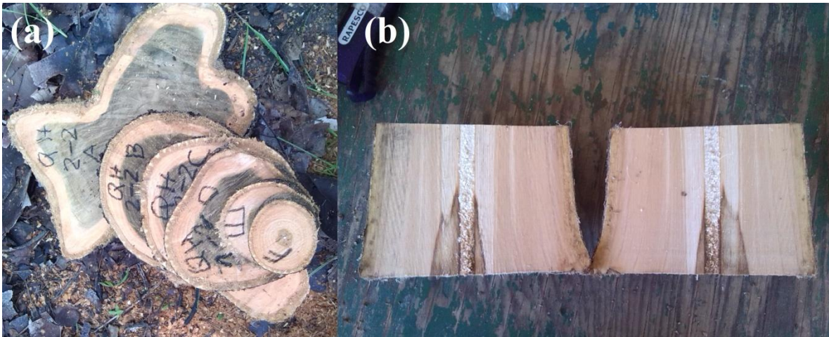
Photo 3: Variation of heartwood across the trunk in Tectona grandis trees of 18 years old (a) and the height at which the heartwood disappears in Tectona grandis trees (b).
