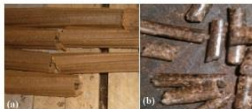
Figure 3 – General aspects of the briquettes (a) and pellets (b) manufactured using coffee pulp.
