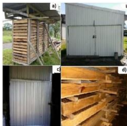
Figure 1 – Devices designed for samples drying: air drying (a); a 6 m 3 capacity solar dryer (b); experimental (conventional) NARDI dryer (c) and stacked trays with gaps to allow air circulation (d).
