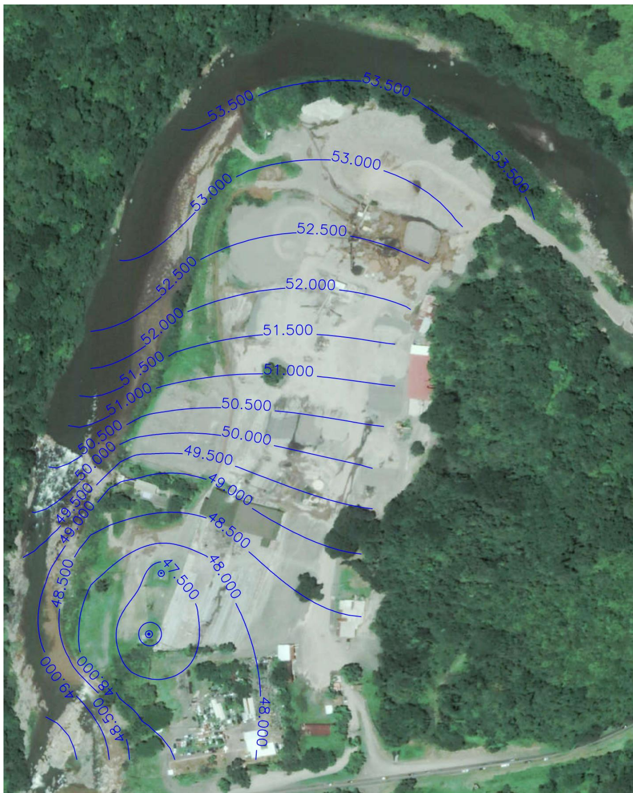
Figure 28 Head contour map for approximated model
