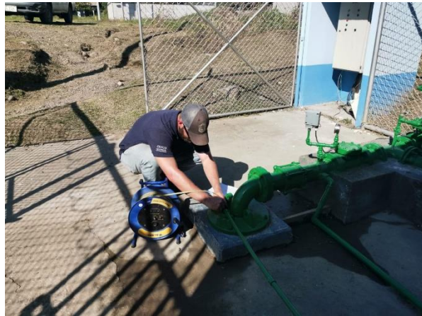
Figure 4 Water level measurements during pumping test
