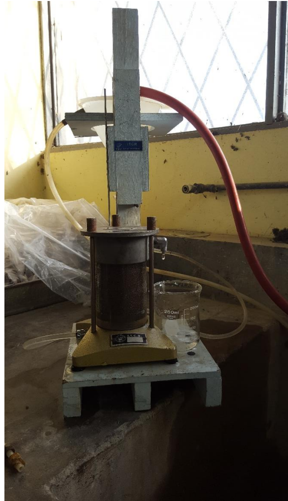
Figure 6 Constant head permeability test
