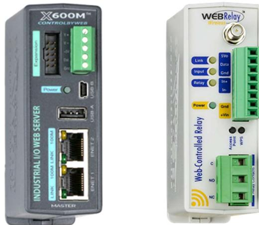
**Figura 3. 6** Controladores X600M y WEB WIRELESS RELAY Fuente: (Control by Web, 2018)
