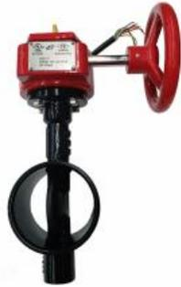
**Specification:** The GD-381FP Butterfly Valve is an indicating type valve designed and listed for use in fire protection systems. This valve is rated for a maximum working pressure of 300 psi (20 bar) and provide a visual indication as to whether the valve is open or closed. It is provided with factory installed supervisory switch monitoring the valve in the open or closed position. Ends are grooved according to ASME B16.1.
